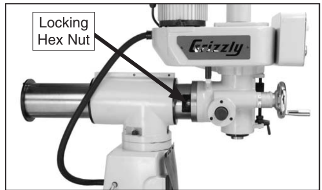
Figure 24. Left side head tilt.
